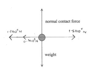
(a) Complete the free-body force diagram to show all the forces acting on the engine.
